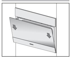
Slide the door onto the hinge guides again. Risk of damage to the door! If the locking clamps are not locked, the door can easily become detached from the hinge guides and be damaged.
