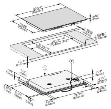
All dimensions are given in mm and inches. The superscript numbers after the cut-out dimensions are the tolerances for the cut-out.
