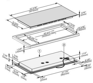
All dimensions are given in mm and inches. The superscript numbers after the cut-out dimensions are the tolerances for the cut-out.
