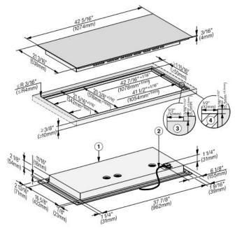
All dimensions are given in mm and inches. The superscript numbers after the cut-out dimensions are the tolerances for the cut-out.
