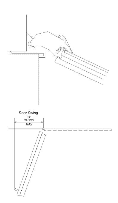
**NOTE**: Additional space needed depending on the thickness of front panels and handle used. **Freezer units cannot be stop pinned at 90°**
