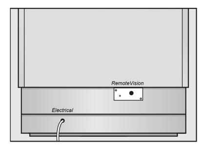
Electrical - 5 foot (1.52 m) - 120 Volt - 15 Amp - NEMA 5-15 molded plug
