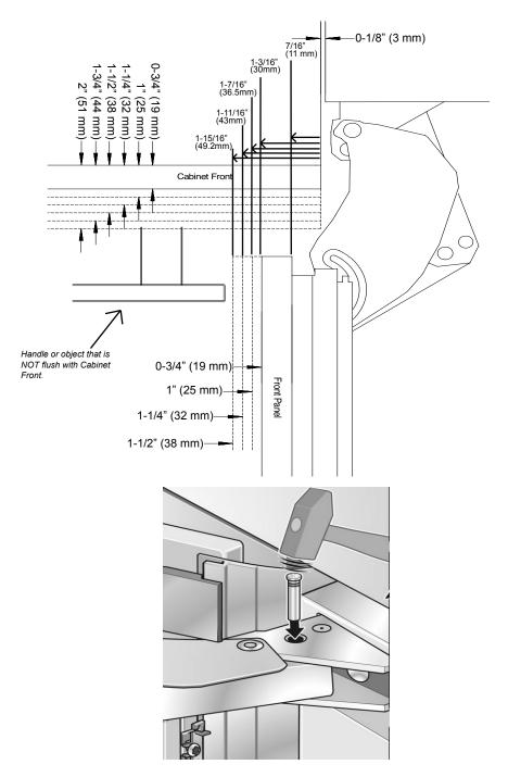
When installing hinge side next to an appliance or object that is within range of the door panel, limit the door opening angle to 90°. This is done by installing the banking pin as illustrated. Insert the banking pin through the holes and drive in with a hammer.
