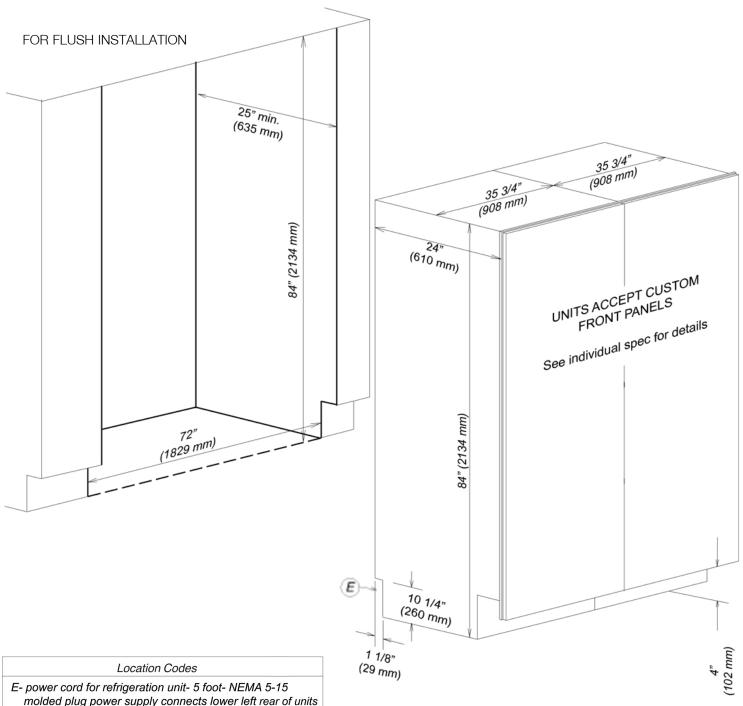
molded plug power supply connects lower left rear of units
