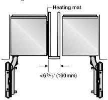
In this case, you will only need the heating mat from the "Merging kit" to avoid condenstaion and prevent damages.
