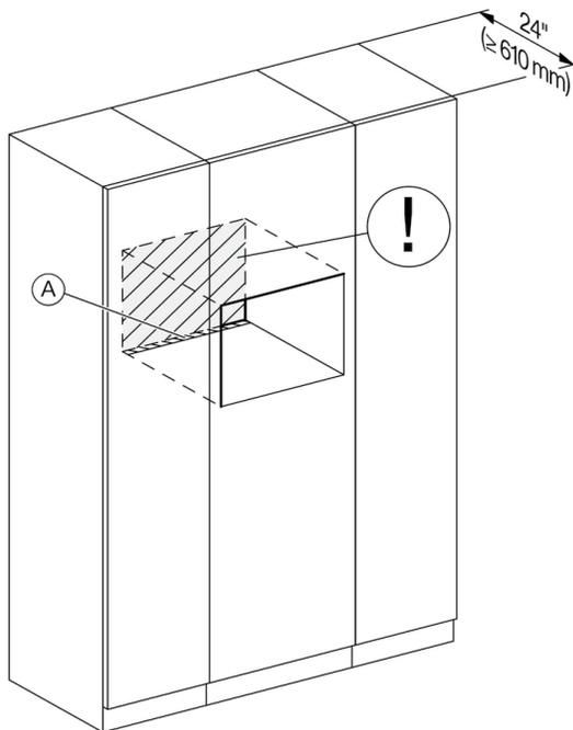
A - Cut-out (4" x 28" [100 mm x 720 mm]) in the bottom of the cabinet for the power cord and Ventilation
