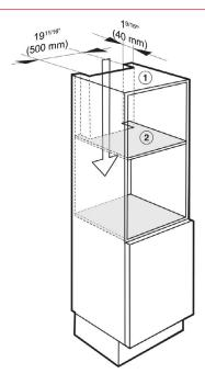
To ensure that the Combi Steam Oven has adequate ventilation, the following cut-outs measuring 19 11/16" x 1 9/16" ( $500 \times 40$  mm) must be made:
