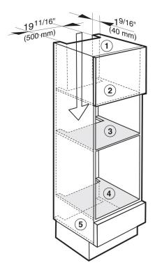
To route the water hoses and to ensure that the Combi Steam Oven has adequate ventilation, the following cut-outs measuring  $19 \, 11/16$ " x  $1 \, 9/16$ " ( $500 \, x \, 40 \, mm$ ) must be made:
