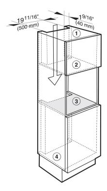
To route the water hoses and to ensure that the Combi Steam Oven has adequate ventilation, the following cut-outs measuring  $19 \, 11/16$ " x  $1 \, 9/16$ " ( $500 \, x \, 40 \, mm$ ) must be made:
