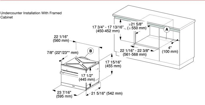
Cut-out (4" x 22" / 100 mm x 560 mm) in the bottom of the cabinet for power  $(\mathbf{A})$ cord and ventilation
