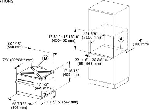
Cut-out (4" x 22" / 100 mm x 560 mm) in the bottom of the cabinet for power  $(\mathbf{A})$ cord and ventilation
